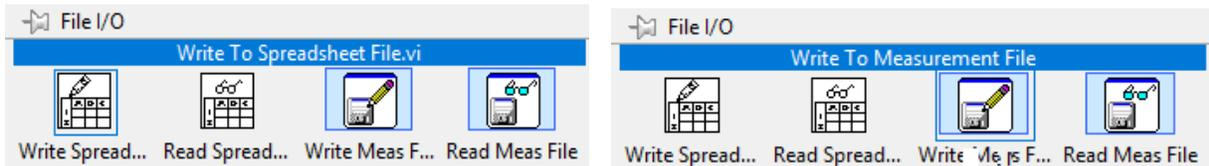
Fig. 3: Funciones "File I/O" Write To Spreadsheet File; Write To Measurement File
